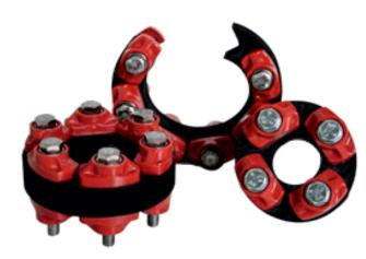
Our Lu-SW building entry consisting of a compact EPDM elastomer ring and flexible segmental pressure plates will save you a lot of time and effort due to its split and custom-fit construction. It can be easily installed subsequent to the installation of the carrier pipe by simply opening the seal insert, putting it around the carrier pipe, inserting it into the core-drilled hole or the wall sleeve, and tightening it. It is not necessary to dismantle the carrier pipe beforehand.
